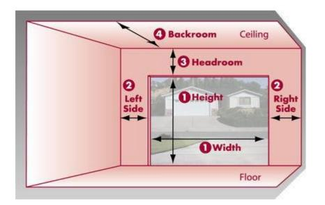
**Step #1 Measure Inside Dimensions of Garage Door Jamb** Measure the width and height of your door opening in feet and inches. This determines the size of door needed. The rough opening measure the same size as the door. Example: If the door size you are wanting is to be 16×7 (width x height), the inside dimensions should be exactly 16' x 7'. A little less is OK. This will make the door rest on the jamb and header on the inside of the door. Width: \_\_\_\_\_\_ Height: \_\_\_\_\_\_
